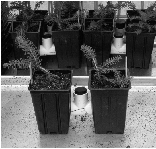
Fig. 1. Two-choice soil olfactometer used in experiments. Larvae were placed in the middle of the "T" tube (PVC pipe) connecting the two pots and allowed 24 h to move.
