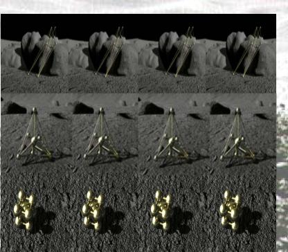
**EMS:** One or more autonomous 12tetrahedral walkers. Rapid (km/day) **locomotion** with many degrees of freedom for navigating inaccessible, rugged terrain: farside, poles, central peaks, debris fields. Reducible in volume for shipping.
