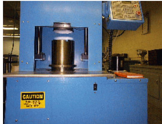
Mold in Compactor Ready to Test
