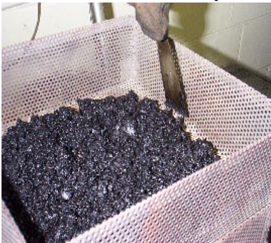
Asphalt Placed in Basket
