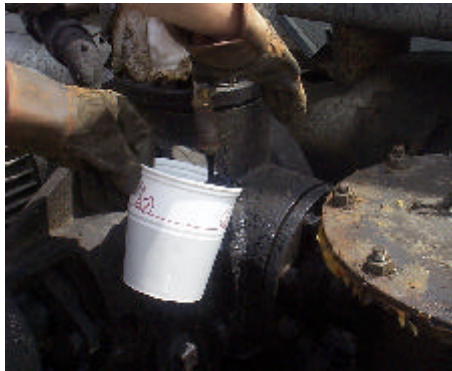
Sampling Asphalt Cement
