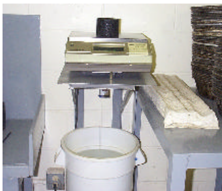
Weighing Specimen to Determine G_{mb}
