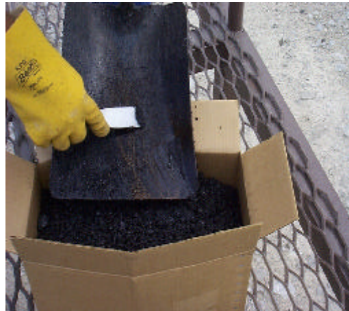
Scraping Sample Off Shovel into Sample Box
