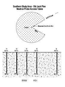
**SSA-YJP**: The neutron probe access tubes were located on a transect line that was N 60 E (true) from the flux tower. Distances from the flux tower were as follows: Tube 1, 50 meters; Tube 2, 70 meters; Tube 3, 75 meters; Tube 4, 80 meters; Tube 5, 85 meters; and Tube 6, 90 meters. All tubes were monitored to a depth of 100 cm and vertical resolution was 10 cm.
