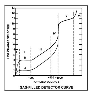
A boron trifluoride  $(BF_3)$  detector (proportional counter) is normally used to monitor only source range core neutron level. How will the detector and source range count rate indication be affected if normal detector high voltage is inadvertently applied during nuclear reactor operation in the power range?
