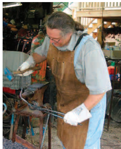
Dana bends a piece of metal rod around the horn of the anvil to make a hook.
