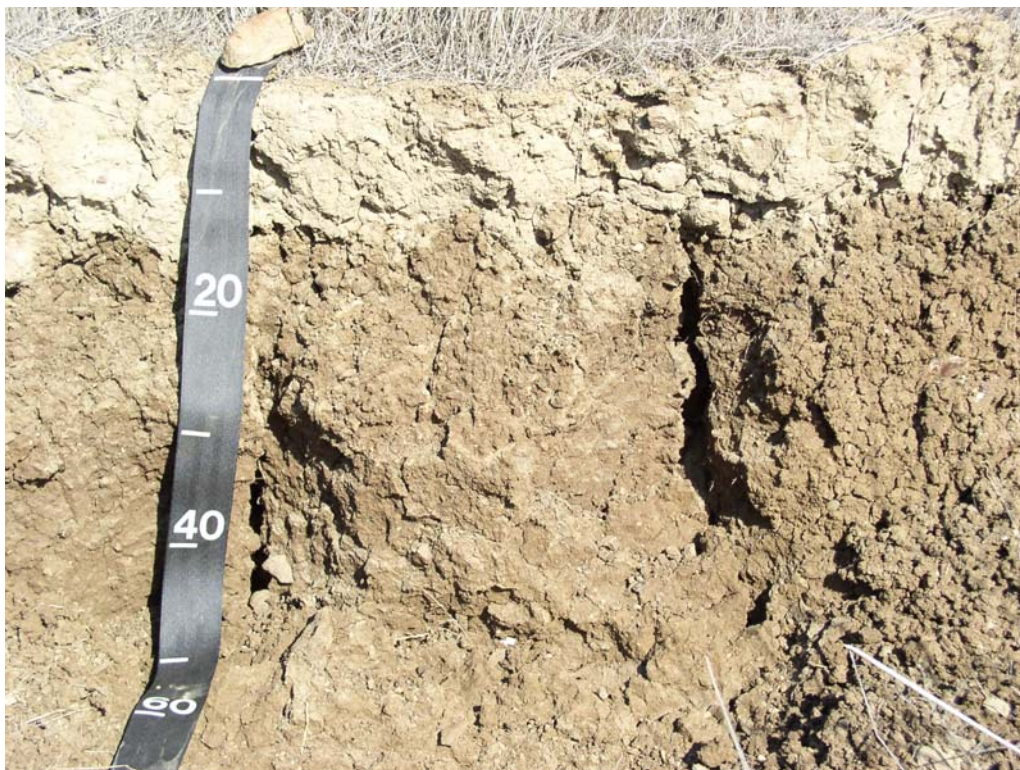
Figure 21.—Typical profile of Luff soils. Currently, these soils commonly support grasslands. Because of the silty eolian mantle, they are highly erosive if the surface is disturbed. On the tape, depth is marked in centimeters.
