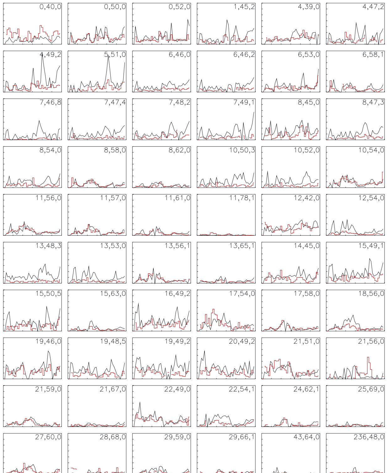
Figure 6. Time series of the modeled and observed sulfate mixing ratios at the 90 locations that had at least 28 observations for the period 17 June to 24 July 1997. The three numbers, i, j, k , at the top right of each panel represent the three-dimensional model coordinates of the location. Model domain is numbered east from the prime meridian (0–360) and north from the equator (0–81), and vertical levels are numbered from the surface.
