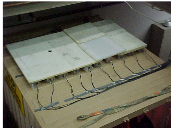
Figure 9. Top detector group with and without borated-polyethylene back shielding.
