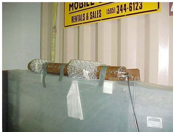
Figure 10. The single INEEL detector positioned on top of the LANL detector.
