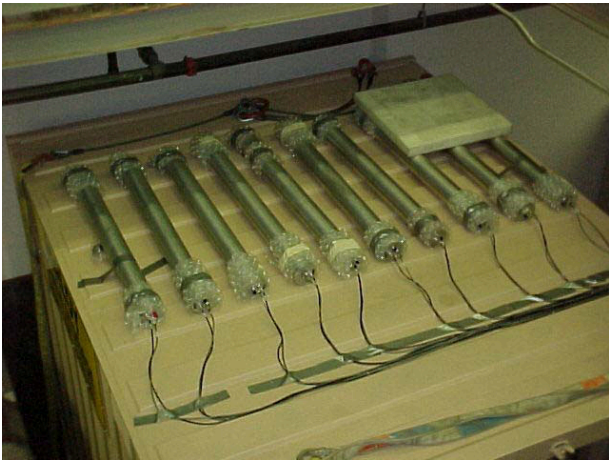
Figure 9. Top detector group with and without borated-polyethylene back shielding.
