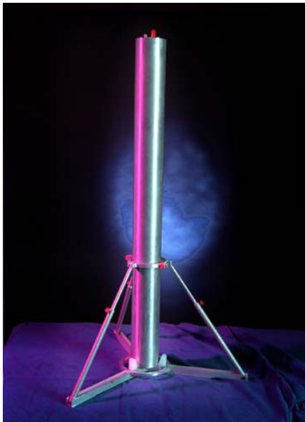
Figure 2. The pulsed photonuclear neutron detector (PPND).
