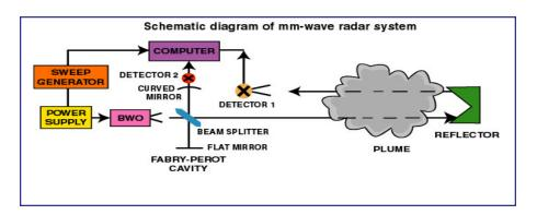
Argonne's system can determine both narrow and broad spectral features of airborne materials at pressures ranging from millitorr to atmospheric and at temperatures from ambient to 300°C. The ability to detect so many substances in such a wide range of conditions makes this mmW radar detection system useful for many types of applications.
