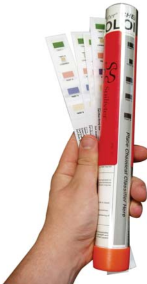
Figure 7. The Spilfyter ® Chemical Classifier test strips and color chart.
