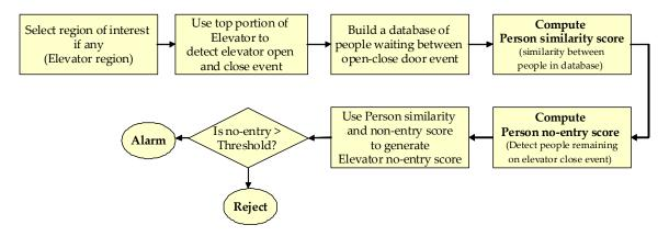
Figure 4. Basic steps of Elevator No Entry Event detection algorithm.
