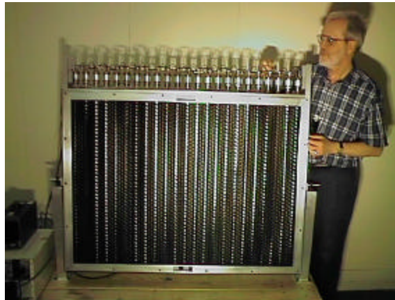
Figure 3.1. Photo of the Completed Square-Meter Moderator-Free Neutron Detection System with ^3\text{He} Tubes, Collimator, Signal Processing Electronics, and Shield. The detector is roughly 10-cm thick.
