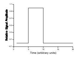
Figure 9. Rectangular envelope for pulse modulation
