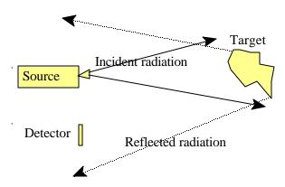
Figure 5. Active imaging system and target
