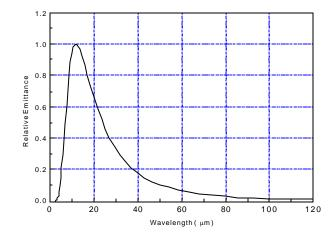
Figure 4. Black-body emittance curve for a body at 37 EC
