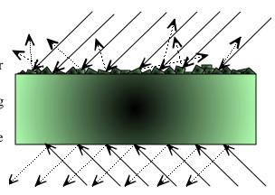
Figure 13. The effect of surface roughness on reflectivity
