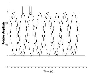
Figure 8. Three sinusoidal waves that are not in phase (in step); the vertical lines help show the degree to which the three waves are out of step and the horizontal lines define the envelope of the waves
