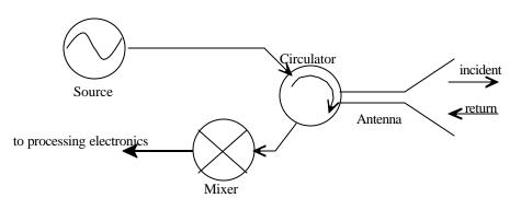
Figure 16. Diagram of an implementation of a cw-Doppler radar system
