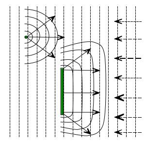
Figure 14. Sketch showing diffraction from an object where the dashed vertical lines indicate the incident waves, the solid lines indicate the reflected waves, and the arrows indicate direction of wave propagation
