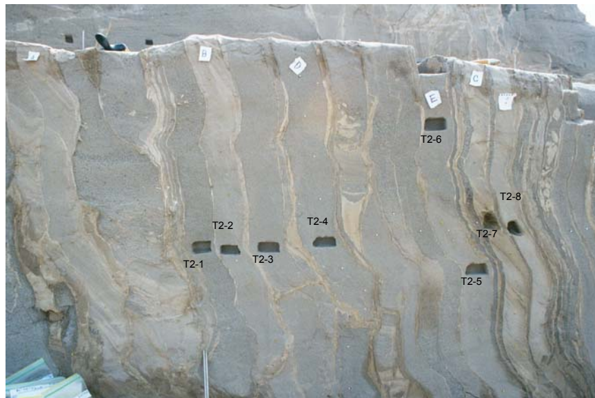
Figure 2.7. Vertical Section of Tier 2 of the Army Loop Road Excavation Showing the Small-Scale Structure of Heterogeneity. Note the vertical and horizontal structures, the fine-textured skins, and the inclusions of varying texture. The rectangular holes are areas where samples were collected for granulometric analysis.
