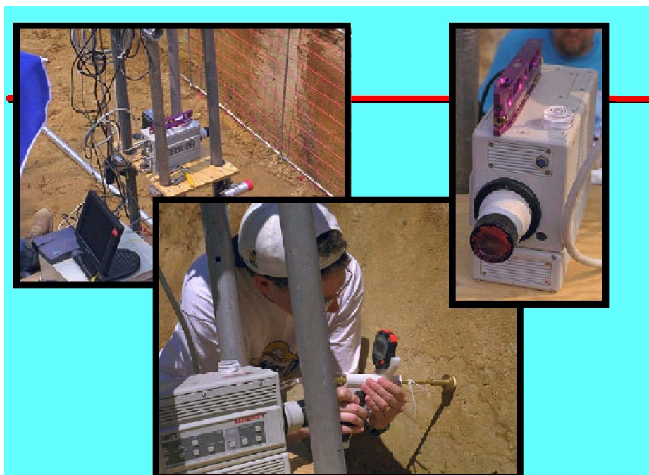
Figure 4.1. Field Setup for High-Resolution Digital Photography and Small-Scale Permeability Measurements
