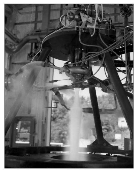
Test of a 5,000-pound-thrust engine used to investigate low cycle thermal fatigue, 4 October 1975. NASA C-75-3125.
