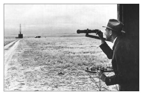
From a safe distance, rocket pioneer Robert Goddard uses a telescope to observe a rocket mounted in a test stand. His left hand rests on the control panel with keys for firing, releasing, and stopping a rocket test, undated, probably the 1930s. Great Images of NASA, http://grin.hq.nasa.gov. 74-H-1245
