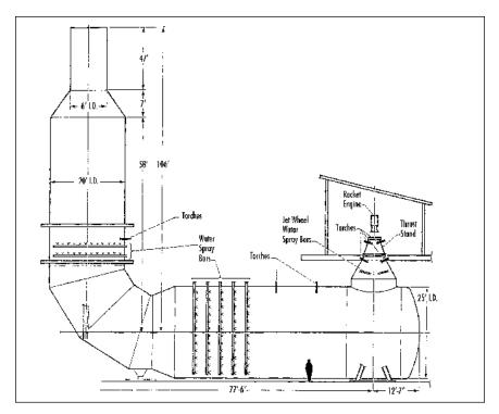
Cross-section of exhaust duct, or scrubber. Five spray bars were located in the horizontal section, with two additional bars in the vertical section. Note the location of the jet wheel in the exhaust duct under the stand and the seven hydrogen torches, used to burn off excess fuel in the scrubber.
