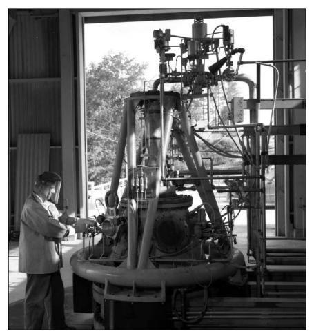
A technician checks the installation of the 20,000-pound-thrust rocket engine on the test stand, October 1957. NASA C-45869.
