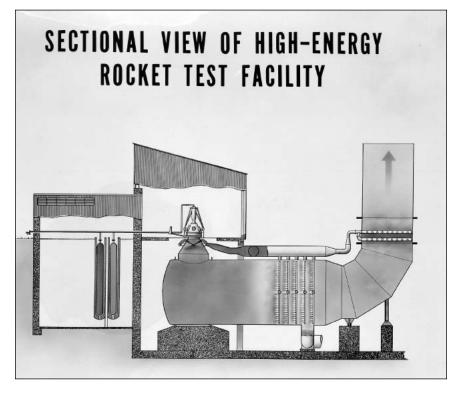
Cross-section showing test stand, scrubber and oxidant pit (left). The scrubber cleansed the exhaust gases and helped to silence rocket engine noise.
