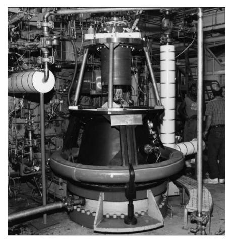
The TRW pintle engine mounted in the RETF test stand, 1993. At a thrust of 40,000 pounds, it was the largest program carried out in the RETF before the facility was shut down in 1995. NASA C-93-6570
