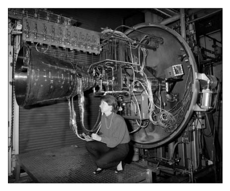
Research engineer Tammy Smith Zurawski performs a final check of a large 1000:1 nozzle prior to testing in Stand B, 1987. NASA C-85-401
