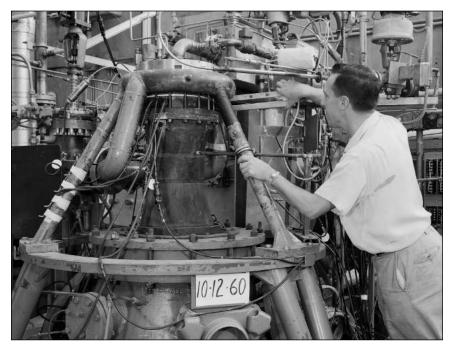
A technician inspects a 20,000-pound-thrust rocket engine used to investigate combustion instability, or screech, October 1960. Screech, a serious problem in rocket engines designed for the Apollo program, was investigated in the RETF using sub-scale models of injectors and thrust chambers. NASA C-54595.
