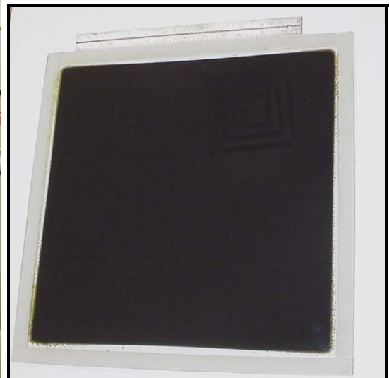
Figure 31: Photograph of a large area CdTe PV film on Pilkington TEC 15 glass, ruler at top is 1 foot long.
