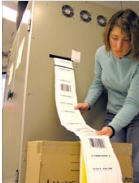
Courtesy of Christina Hammock / Special to The Antarctic Sun Christina Hammock gathers data coming out of Palmer Station’s Radionuclide Aerosol Sampler/Analyzer in the TerraLab.
