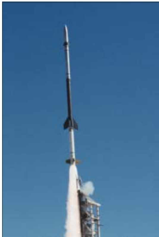
A Terrier-Black Brant sounding rocket of the type that will carry SUMI above Earth's atmosphere.
