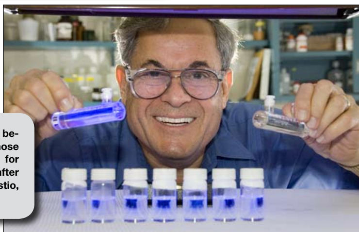
Richard (Dick) Hahn with samples of gadolinium-loaded liquid scintillator (LS), that he and his BNL colleagues, Minfang Yeh and former postdoc, Alex Garnov, have developed as antineutrino detectors. The blue samples on the table and in Hahn's right hand contain fluorescing compounds in order to shift the emitted light into the blue region, so it can be easily detected. The colorless sample in his left hand does not contain the wavelength shifter.
