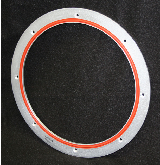
Figure 2.—Photograph of a test specimen showing the front side with a single seal.
