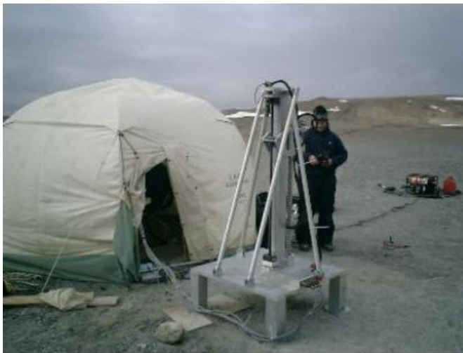
Figure 11. 20-kg Mars prototype drill tested with vibration sensors in Haughton Crater on Devon Island, Nunavut, Canada
