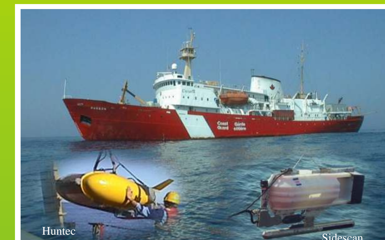
Two instruments used in the acquisition of seismic data, the Huntec and the Sidescan
