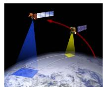
formation flying requires precise navigation. EO1 must know its velocity, position, and the exact time in order to maintain its position with respect to Landsat and to precisely point its imaging instruments.
