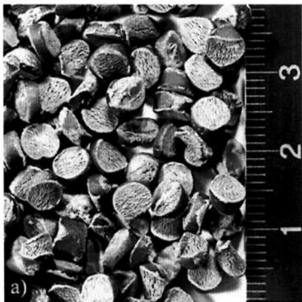
Fig. 10 a) Granulate: PP-BaSO 4 , d_{sl} = 4 mm, \rho_{sl} = 2.64 g/cm 3 and b) granular slide profile scanned with a laser distance sensor orthogonal to ramp at location x = -67 m and z = 67 m.
