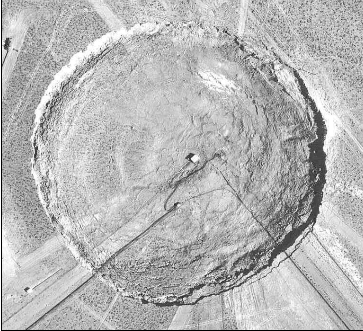
Figure 5—Aerial photograph of collapse sink at Portmanteau (U-2ax) detonation site, Yucca Flat, Nevada. Portmanteau was detonated on August 30, 1974. This photograph was taken seven days later on September 6, 1974. Note the distinctive edge of the collapse sink and presence of surface materials that subsequently slumped into the sink at its perimeter.
