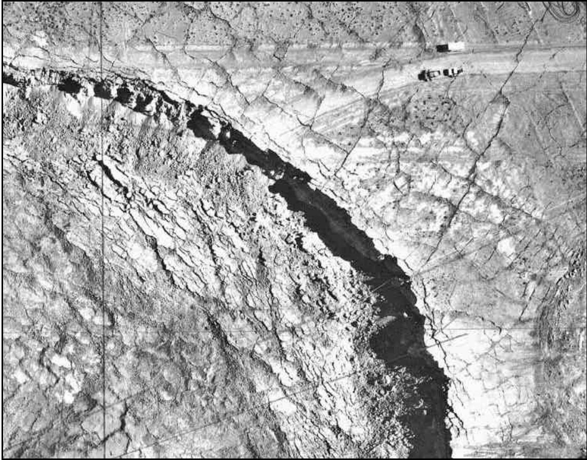
Figure 6—Aerial photograph of collapse sink at Commodore (U-2am) detonation site, Yucca Flat, Nevada. Commodore was detonated on May 20, 1967. The distinct edge of the sink and the occurrence of radial and concentric cracks extending from its perimeter are prominent surface effects at this site. Note the two trucks on the “truncated” dirt road at upper right.
