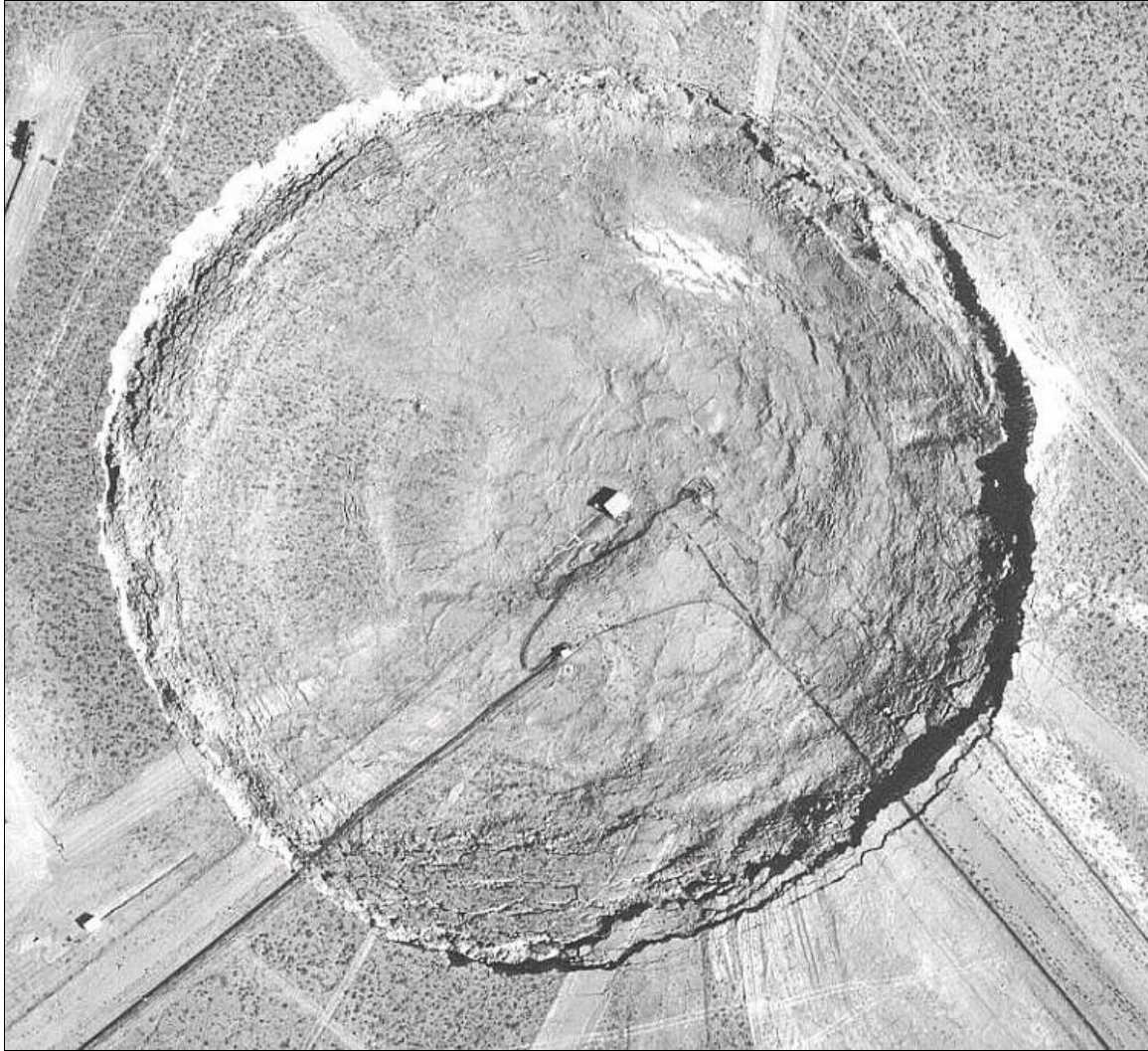
Figure 5—Aerial photograph of collapse sink at site U-2ax, Yucca Flat, Nevada. Portmanteau was detonated on August 30, 1974. This photograph was taken seven days later on September 6, 1974. Note the distinct edge of the collapse sink and presence of surface materials that slumped into the sink at its perimeter following surface collapse.
