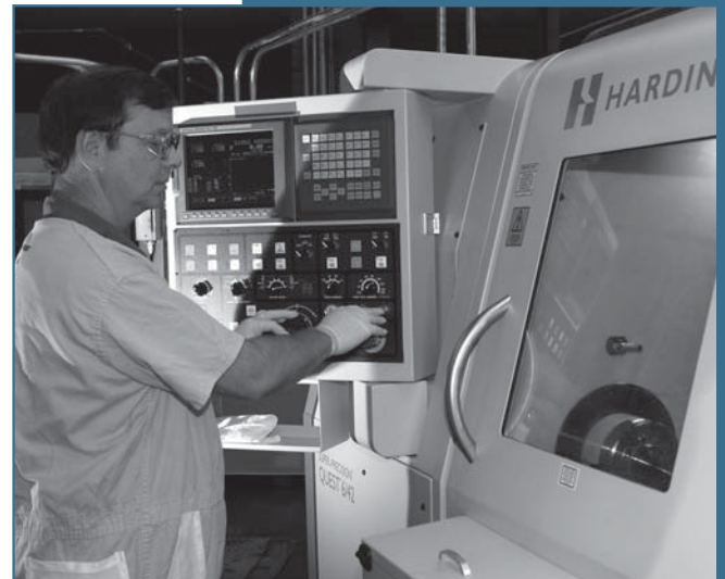
Y-12 machinist Mark Sherrod works with the new efficient, high-precision Hardinge lathe.
