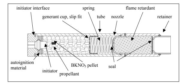
Figure 1. Final design of gas generator housing configuration.
