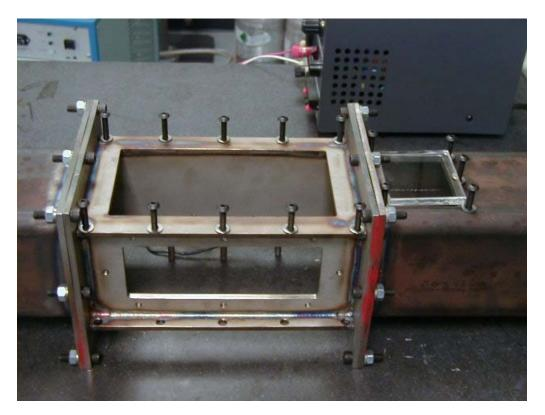
Figure 5. Photograph of burner section.
