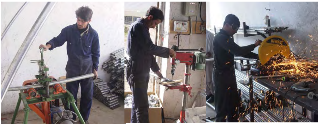
At the Workshop at PAC, sawing (cutting), drilling and pipe bending machines are in action to manufacture GH pipes.
