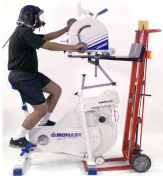
Dual-Cycle Ergometer used for Exercise-Enhanced Prebreathe
