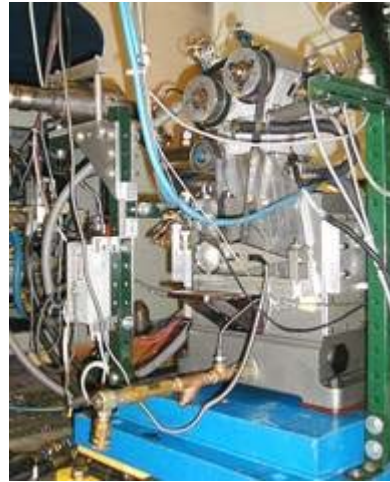
UM Heat Transfer Engine (Thermal Management)
