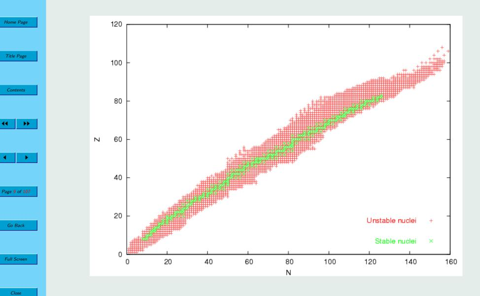
Nuclei with measured masses according to 2003 AME. NOT shown: nuclei for which quoted mass is an estimate based on local systematics (indicated by # in table).
