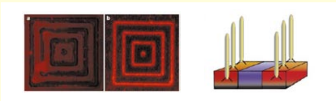
Selection of peptides with semiconductor binding specificity for directed nanocrystal assembly [42].
