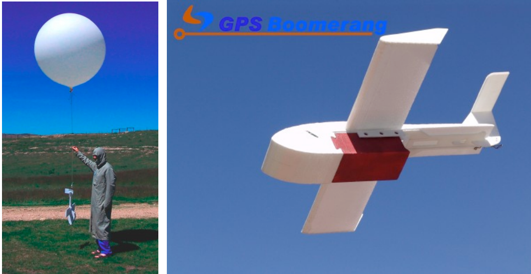
Fig. 1. The “DataBird” glidersonde produced in New Zealand by GPS Boomerang. Launch configuration (left), the glider as it approaches to land (right). Red box is counterweight used when a radiosonde is not carried. Both images from GPS Boomerang web site at: http://www.gpsboomerang.com/
