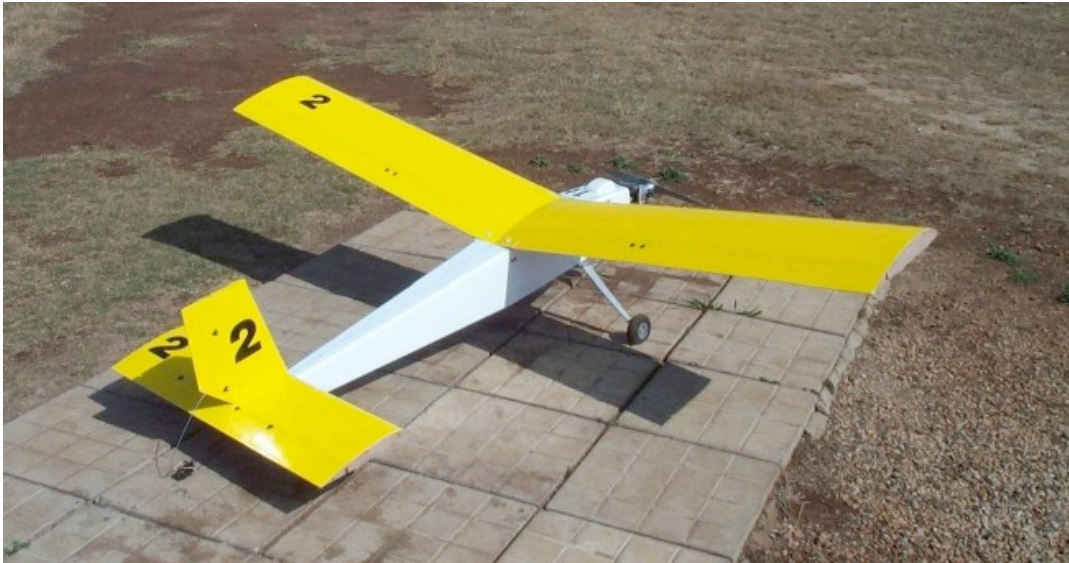
Fig. 2. Prototype powersonde in South Africa with gasoline engine and fiberglass body. Otherwise very similar to a number of model airplanes.
