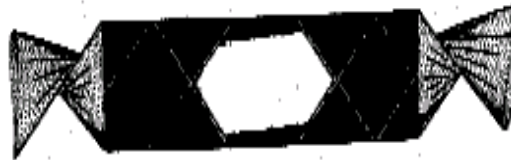
Example of a design for packaging that shows a twist type closure.
