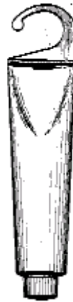
Example of a design for packaging a tube with a crimped end with a hanger.
