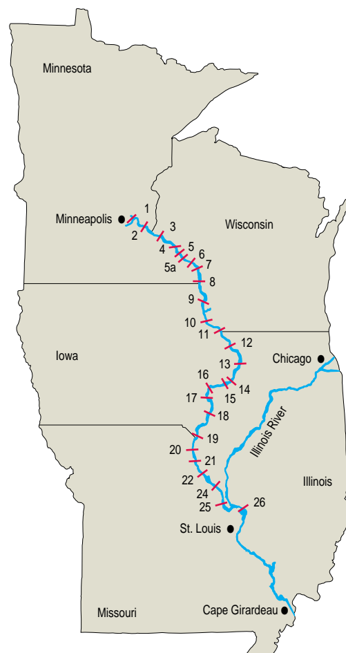
Fig. 1. The Upper Mississippi River. Numbers indicate reservoirs formed by navigation dams and known locally as pools.
