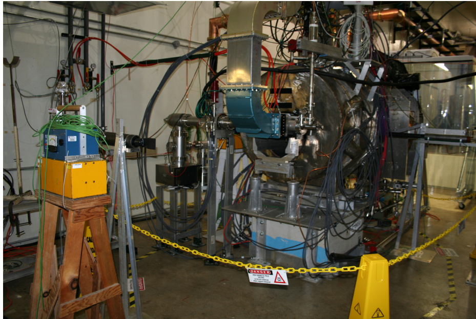
Current Picture of the MTA Hall showing the 5 T magnet in the foreground and the waveguide RF power input to 805 MHz cavity in back ground is the 201 MHz cavity.
