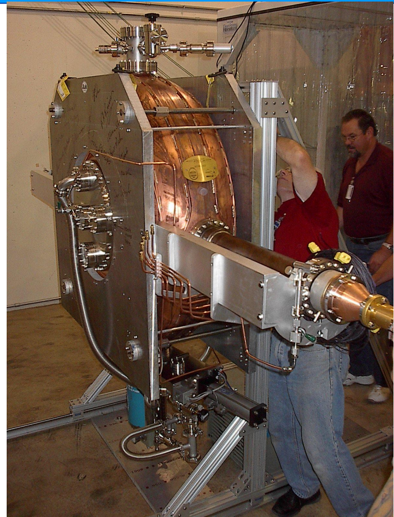
201 MHz cavity during preparation for installation in Aug 05.
