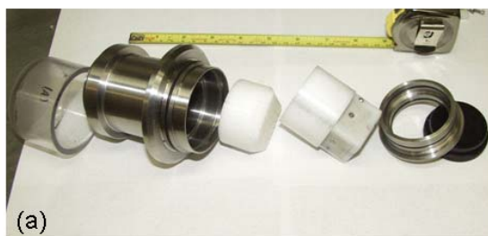
Figure 5. Sample holder and components form directional permeability measurements using the UFA, (a) UFA sample holder, (b) cube insert for UFA sample holder.
