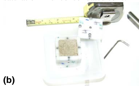
Figure 5. Sample holder and components form directional permeability measurements using the UFA, (a) UFA sample holder, (b) cube insert for UFA sample holder.
