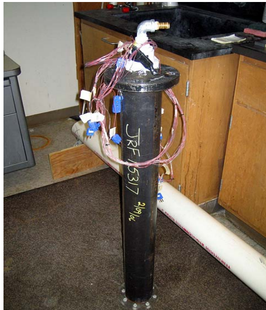
Fig. 6 Prototype pipe with thermo couples.
