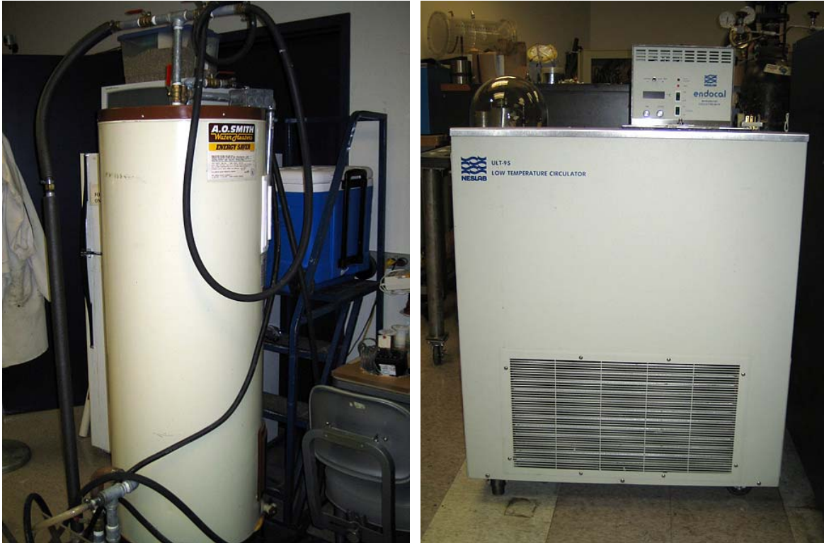
Fig. 10 Hot Water Heater(left) and Low temperature Circular(right).
