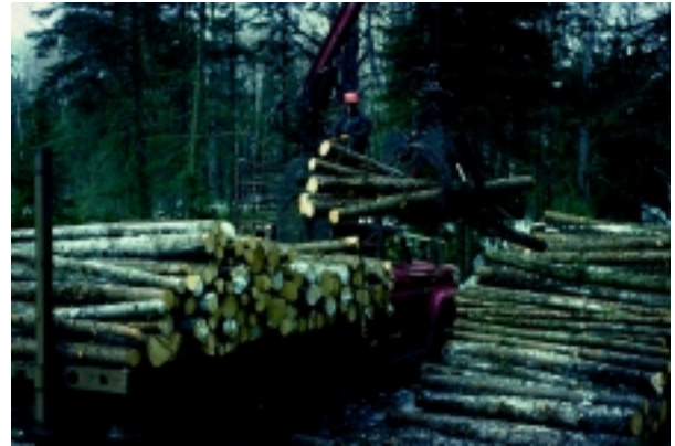
Figure 6: Loading logs on the truck for transport to the milling plant; Superior National Forest, Minnesota; photo from USDA Forest Service.
