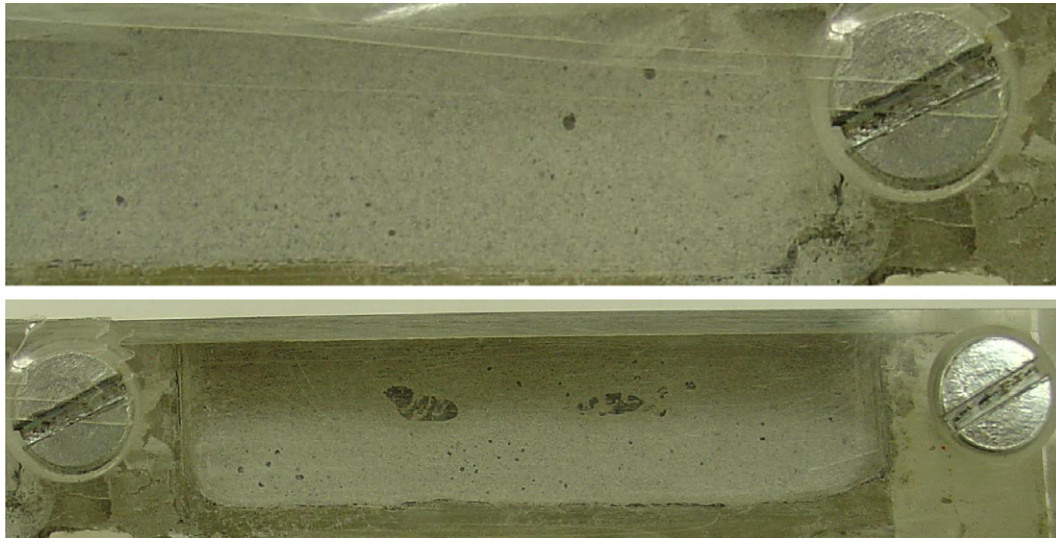
Fig. 7. Photographs of side edges of sealed (top) and exposed to drying at its top surface (bottom) tile adhesive specimens at the end of experiment #9. Two “eye-shaped” voids (dark) several mm in size can be seen in the middle of the specimen exposed to the drying environment.
