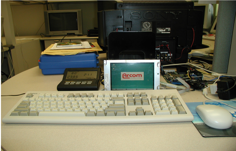
Fig. 3. The SBC MediaGX board with the flat-panel display, keyboard and mouse. The flat-panel display is the one with the Arcom logo. The Davis Instrument is to the left of the display.
