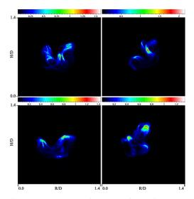
Fig. 3. Instantaneous horizontal soot images in a 7.1 cm methane flame at H = 0.5D. The color bar denotes arbitrary units.
