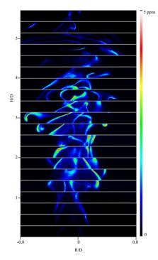
Fig. 2. Collage of instantaneous images of soot volume fractions in a 7.1 cm methane flame.
