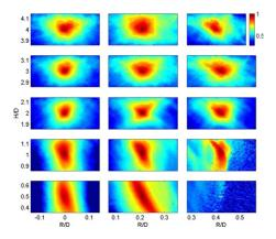
Fig. 7. SCC of soot volume fractions in a 7.1 cm methane flame.
