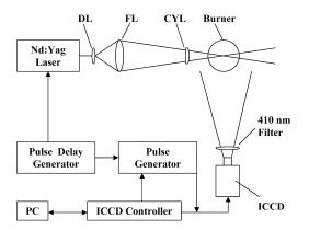
Fig. 1. Plan view of the experimental system.
