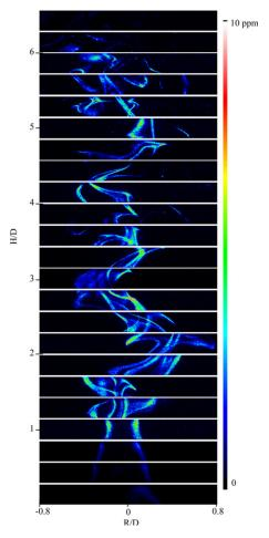
Fig. 8. Collage of instantaneous images of soot volume fractions in a 7.1 cm ethylene flame.
