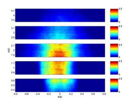
Fig. 4. Averaged soot volume fractions in a 7.1 cm methane flame. The color bar denotes ppm.
