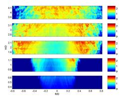
Fig. 5. Fluctuation intensities of soot volume fractions in a 7.1 cm methane flame.
