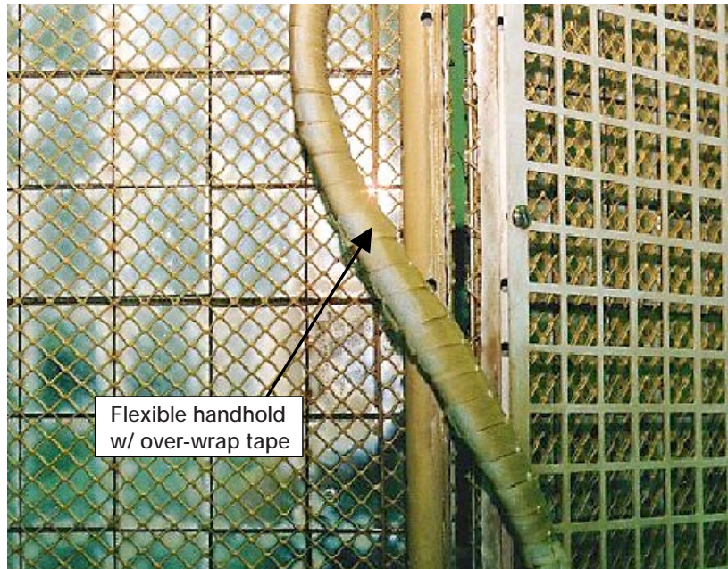
Figure 5. Close-up of a flexible handhold showing the over-wrap tape (ref. 2).
