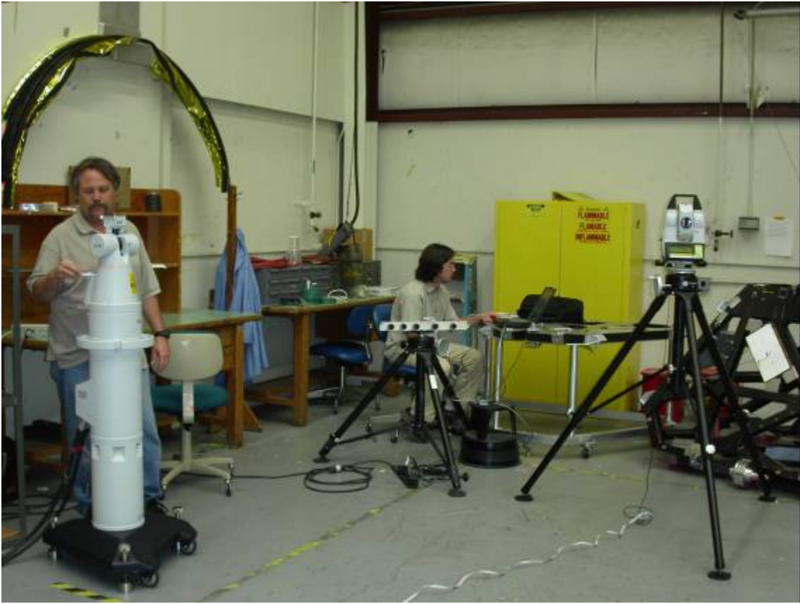
Figure 1. Camera calibration experimental setup with a laser tracker (left), a total station (right), and a stereo camera-head with firewire cables and a laptop computer (center)
