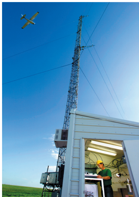
The ARM Carbon Project in Oklahoma is one of the world's best-equipped sites for carbon studies, using a variety of instruments mounted on the ground, in towers, and in aircraft to measure a variety of interactions among soils, plants, and the atmosphere.
