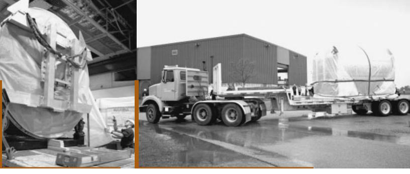
The Central Outer Tracker is loaded onto a special low-riding, air-suspensioned flatbed truck from its assembly site in Industrial Center Building 4 (left), covered to protect it from the elements (center), and wheeled outside to prepare for its journey across D Road to the CDF Assembly Hall (right).
