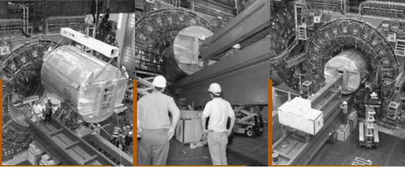
The COT is lowered into position on the siege cart (left). Mukherjee likens the siege cart (center) to a "battering ram," but its job is to coax the COT into the center of the big CDF detector (right). Technicians stationed inside the big detector (below) guided the COT into position with only two millimeters of radial clearance. They were able to make adjustments in both the siege cart and the "H-frame" to avoid contact.
