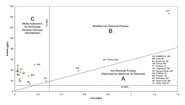
Figure 2-1. Arsenic Treatment Selection Guide as a Function of Initial Arsenic and Iron Content of Water (Sorg, 2002)
