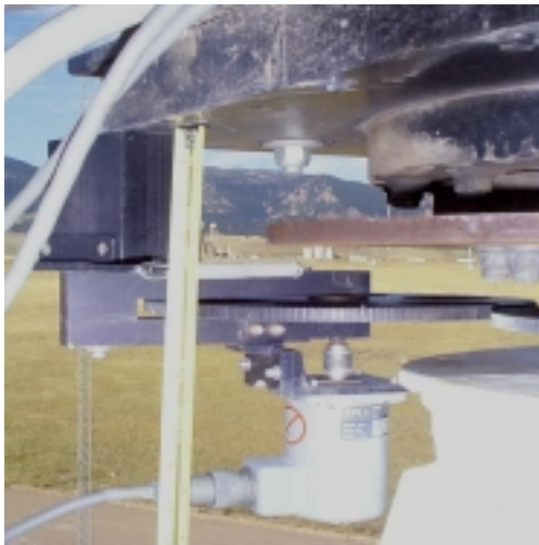
Figure 39. Yaw angle encoder photograph and orientation
